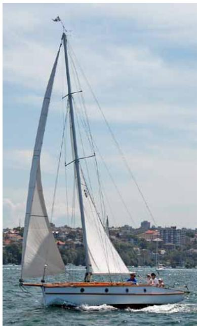
**DIMENSIONS:** 32 feet long (hull), 11 feet beam, 5' 9" draught, lead keel.
