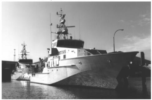
These vessels will form an integral part of the Australian Customs **DECEMBER** 99 Service fleet of patrol vessels and will complement Customs Coastwatch aircraft which provide a national civil surveillance and response service. The 38 metre aluminium hulled patrol boats have a range of 1000 nautical miles at 20 knots and are capable of operating around Australia's 37.000 kilometre coastline and out to the edge of the 200 nautical mile Exclusive Economic Zone.
