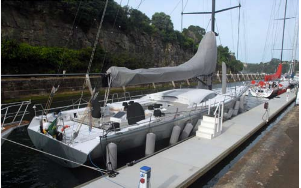
The Farr-designed McConaghy-built maxi Leopard 3 lying at rest astern of Wild Oats XI in Woolwich Dock before the start of the 2007 Sydney to Hobart yacht race. The remarkable yacht has a rig which towers 47 m above the water and can carry some 1378 square metres of sail. Her canting keel is said to be equivalent to 200 crew members sitting on the rail and it is canted by two hydraulic rams with a maximum force of 61 t!
