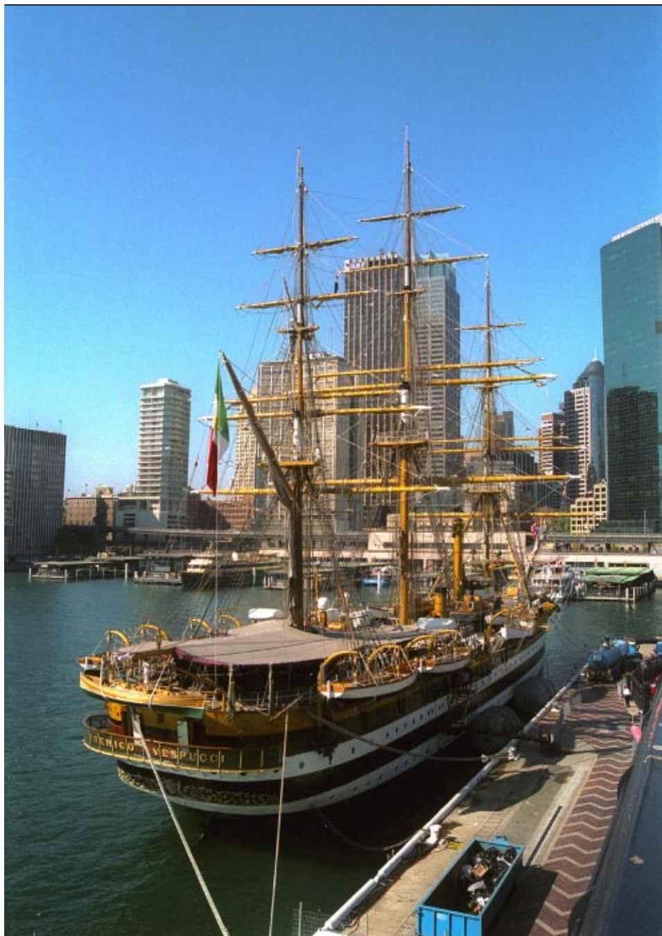
The Italian Navy's sail training ship Amerigo Vespucci during her recent visit to Sydney. Built in 1931, the steel-hulled ship displaces 4,221 tonnes and has a sail area of 2,100 square metres. The ship is used by the Naval Academy and has a complement of 243 including 150 trainees.
