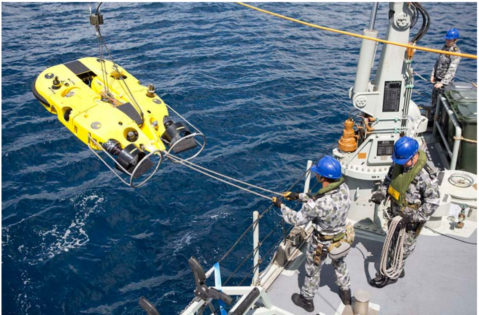
Able Seaman Combat Systems Operator Mine Warfare Ryan McDonald (right) and Seaman Combat Systems Operator Mine Warfare Rodney Burnett guide the Mine Disposal Vehicle outboard from HMAS Yarra to investigate an underwater sonar contact in the waters of Papua New Guinea
