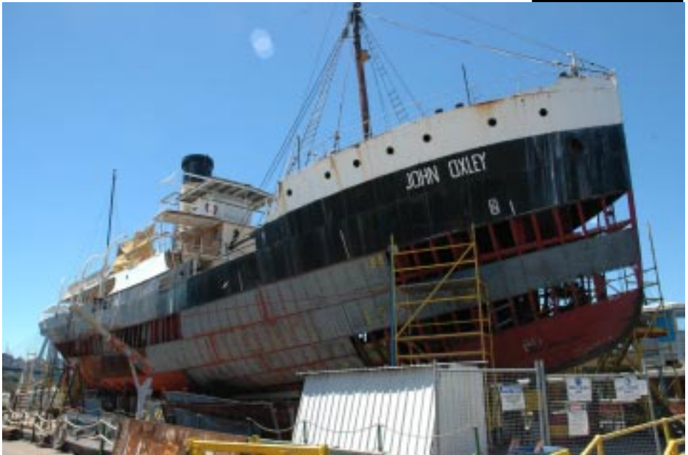
The dedicated volunteers of the Sydney Heritage Fleet have been making progress with the restoration of the 1927-built John Oxley . Large areas of new shell plates can be seen in the photo above. Recent work has included replacing floors under the boilers through access holes in the shell (below)
