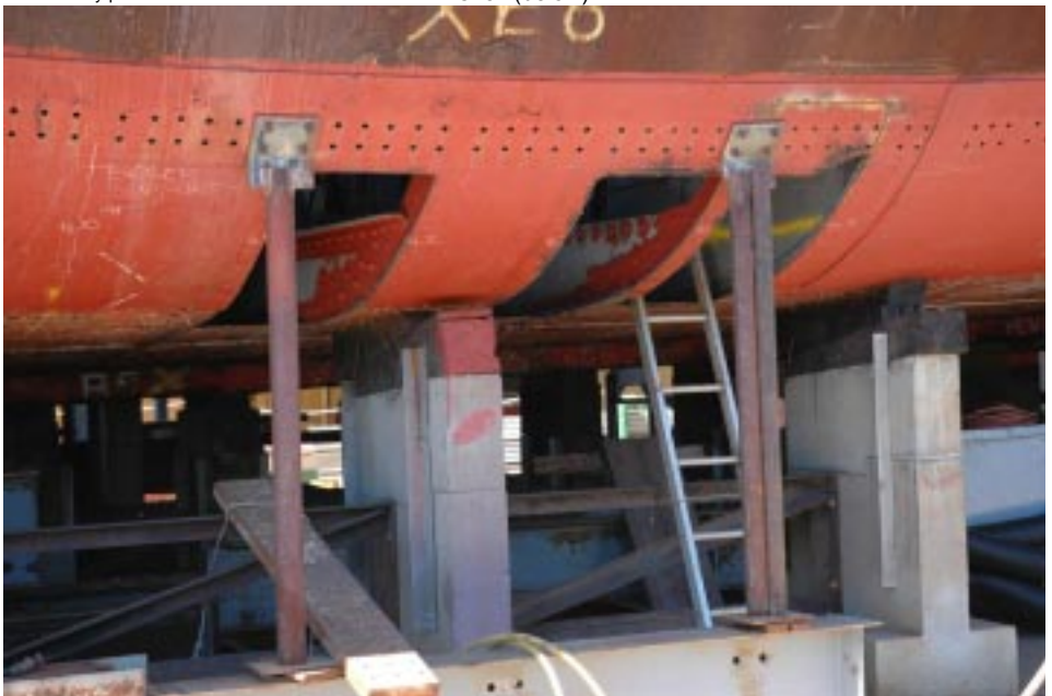
The dedicated volunteers of the Sydney Heritage Fleet have been making progress with the restoration of the 1927-built John Oxley . Large areas of new shell plates can be seen in the photo above. Recent work has included replacing floors under the boilers through access holes in the shell (below)
