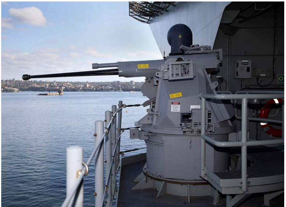
One of the four 25 mm Typhoon guns fitted on board HMAS Canberra
