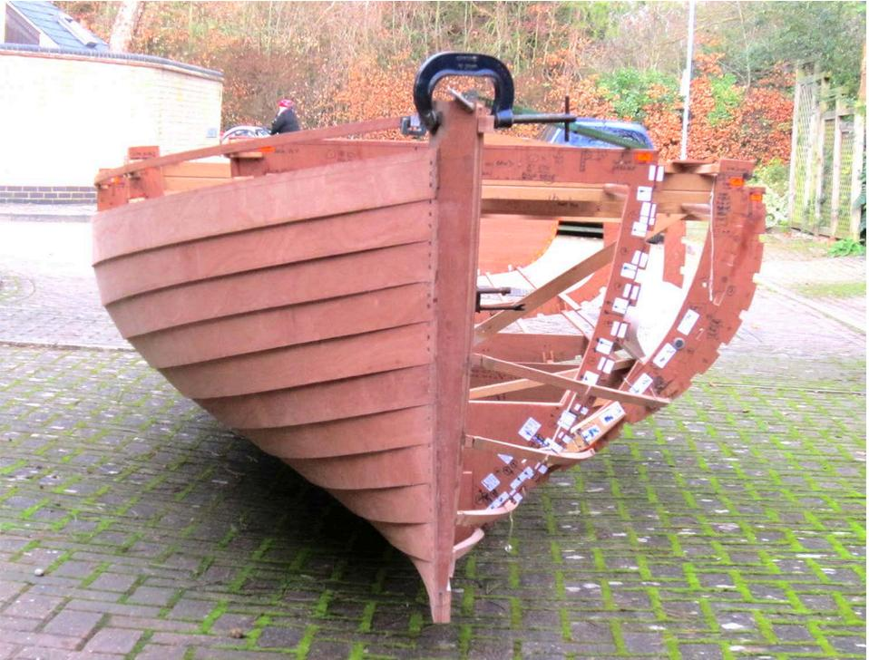
Figure 1: The half-planked hull in 2021. I decided to do the starboard side first, so any errors in setting-out would only need to be corrected once. This did not distort the hull.
