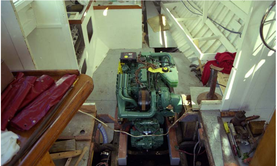
In August 1999 Captain Amora had a major refit when the original venerable BMC six-cylinder diesel engine was replaced by the Volvo diesel she has today
