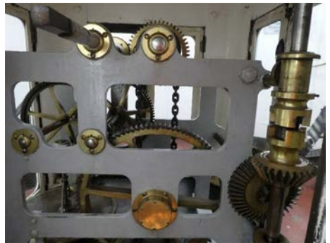
Governor, gears and clutch for the light mechanism
