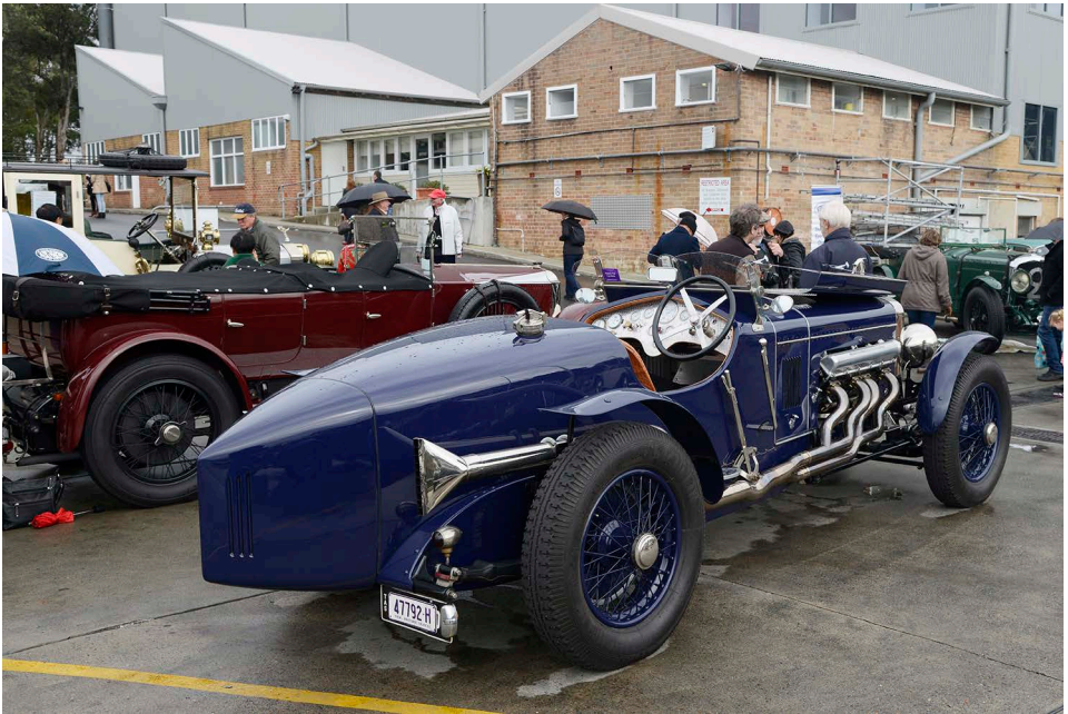
The Hispano-Suiza-engined Delage was fitted with an 18 L aero engine
