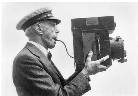
Pioneer: The original mouth-operated Beken camera
