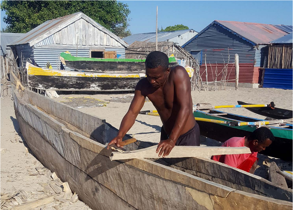
A local shipwright shaping a gunwale plank
