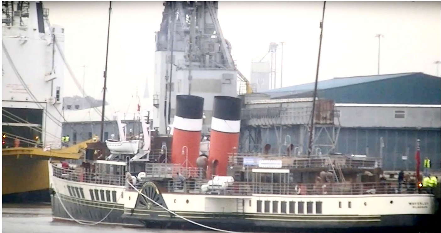
Fig.1 shows her alongside, parallel to the quay. The crew are passing a long hawser aft to a bollard on the quayside. The slack will then taken up using the steam winch on the foredeck.
