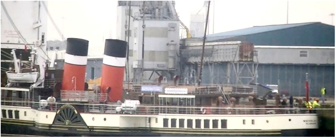
In Fig. 2, the hawser has been put into tension with a Dead Slow Ahead on the engine. As this occurs, the hull rotates, with the stern coming into contact with the quay and the stem moving away from the quay. She then starts to rotate around the contact point between her stern and the quay and the bow comes out further. The crew on the steam winch start to control the free length of hawser to make sure that the stern stays in the same position. The tension is kept up by using the engine."
