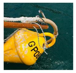
The method of joining the clip to the buoy, with the mooring clip on the boat hook. Easing the white rope allows the clip to slide off the boat hook and close.
