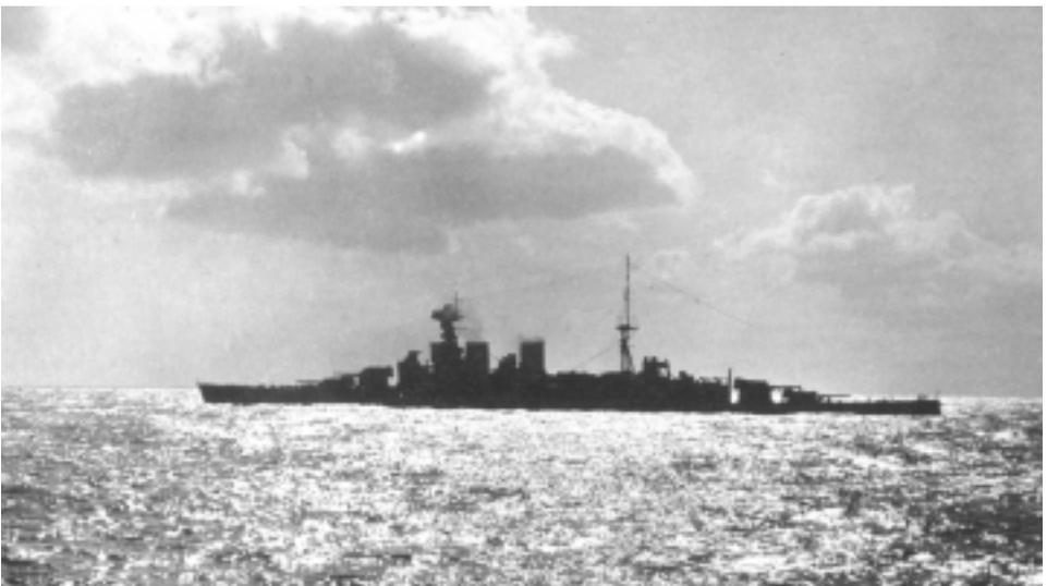
32.07 knots. She was armed with eight 15-inch guns, twelve 5.5-inch guns, four 4-inch guns and six 21-inch torpedo tubes.
