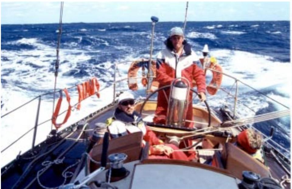
for the Lord Howe. A113 is built strong and heavy. The displacement hull and robust masthead rig make her both powerful and seakindly. But she does have some notable eccentricities. There are 13 winches for the rig, but just two cleats.
