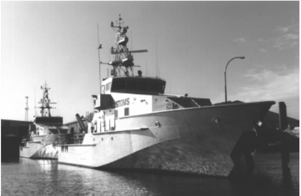
These vessels will form an integral part of the Australian Customs Service fleet of patrol vessels and will complement Customs Coastwatch aircraft which provide a national civil surveillance and response service. The 38 metre aluminium hulled patrol boats have a range of 1000 nautical miles at 20 knots and are capable of operating around Australia's 37,000 kilometre coastline and out to the edge of the 200 nautical mile Exclusive Economic Zone.
